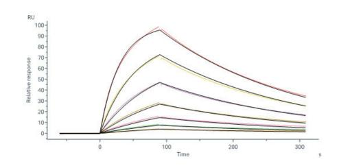
Anti-SEZ6 antibody captured on Protein A Chip can bind Biotinylated Human SEZ6 Protein, His,Avitag (Cat. No. SE6-H82E3) with an affinity constant of 40.6 nM as determined in a SPR assay (Biacore 8K) (Routinely tested).
