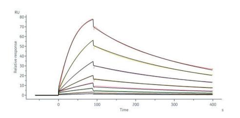
Biotinylated Human IL-18 R1, Fc,Avitag (Cat. No. IL1-H82F9) captured on Protein A Chip can bind Human IL-18 Protein, premium grade (Cat. No. IL8-H5114) with an affinity constant of 14.2 nM as determined in a SPR assay (Biacore 8K) (Routinely tested).
