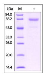
Mouse Glycophorin A, Fc, His Tag on SDS-PAGE under reducing (R) condition. The gel was stained overnight with Coomassie Blue. The purity of the protein is greater than 95%.
