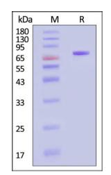
Human Transferrin R, His Tag on SDS-PAGE under reducing (R) condition. The gel was stained with Coomassie Blue. The purity of the protein is greater than 95% (With Star Ribbon Pre-stained Protein Marker).
